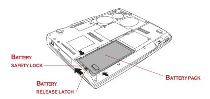
Figure 6-1 Releasing the battery pack
